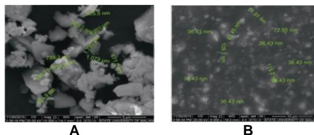
**Figure 1.** The result of SEM of MTA and NMT (A) SEM result of MTA showed the average MTA particle size was 0.508 µm (15000x magnification). (B) SEM result of NMT showed the average NMT particle size was 75.8 nm. (8000x magnification).
