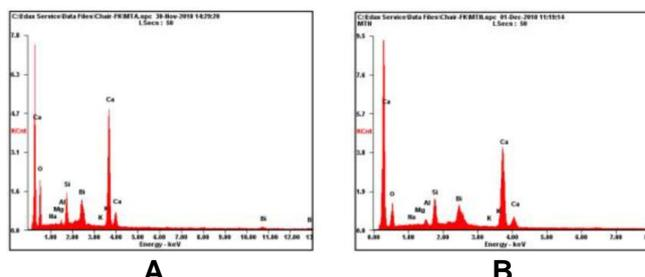
**Figure 2.** The result of EDAX of MTA and NMT (A) EDAX result of MTA showed that the quantity of calcium was the highest, followed by oxide, bismuth, and silicate. (B) EDAX result of NMT showed that the quantity of calcium was the highest, followed by silicate, oxide, and bismuth respectively.
